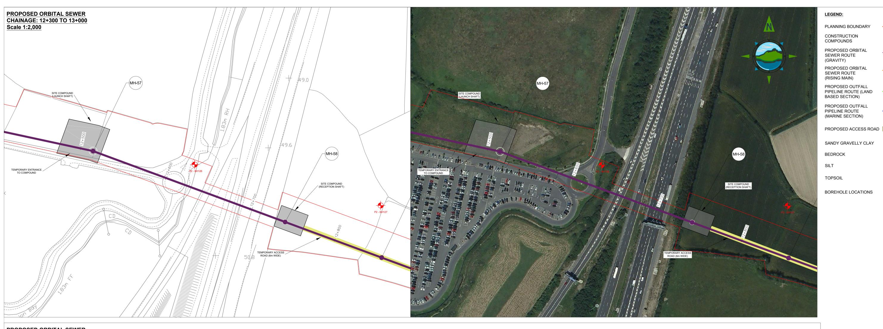
PROPOSED ORBITAL SEWER CHAINAGE: 12+300 TO 13+000 Scale H-1:1,000 / V-1:100 9.0mØ LAUNCH SHAFT P2 - BH126 , 5.5mØ RECEPTION SHAFT P2 - BH127 –1800mmØ TRŒNCHLESS CROSSING– -1,800 mm Gravity Sewer-Pipe &Ground Condittions -Grassland-—M1 Motorway and Roundabout— -Grassland-**Ground Level** Invert Level 12+400 12+500 12+600 12+700 12+800 12+900
