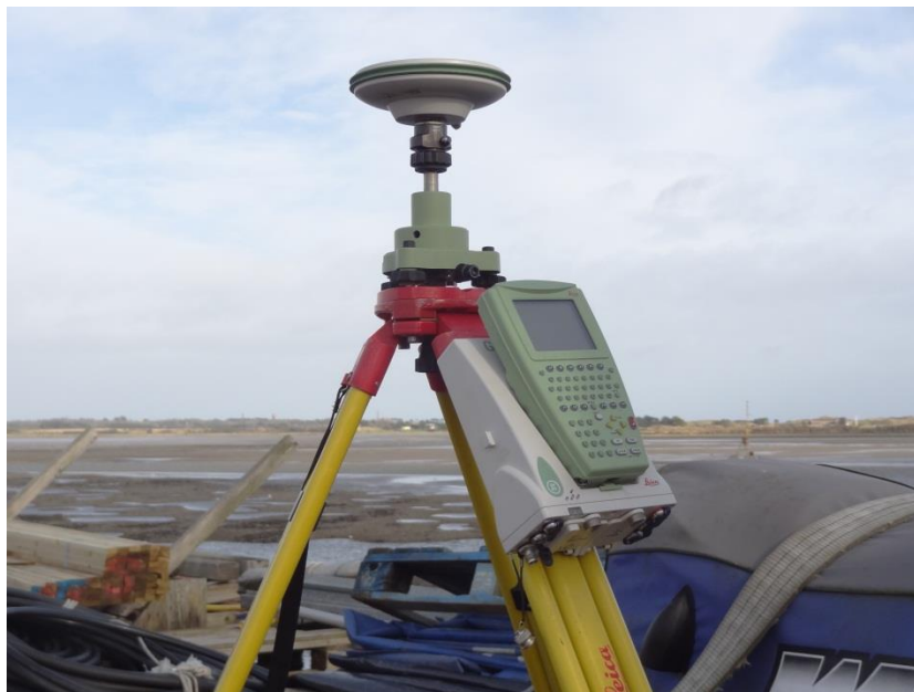
Figure 42 - The GNSS system mounted on the Tripod
