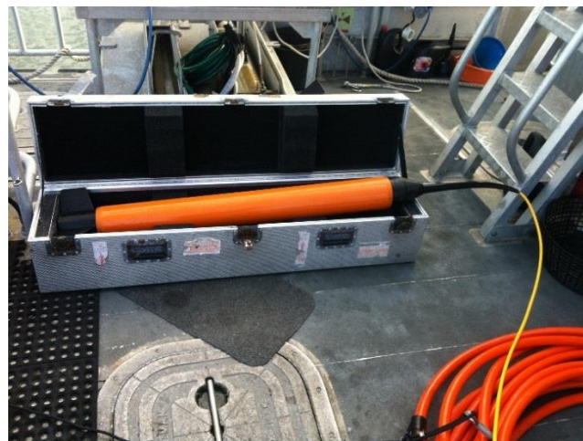
Figure 57 - The Marine Magnetics SeaSPY magnetometer on the deck of the RV Keary
