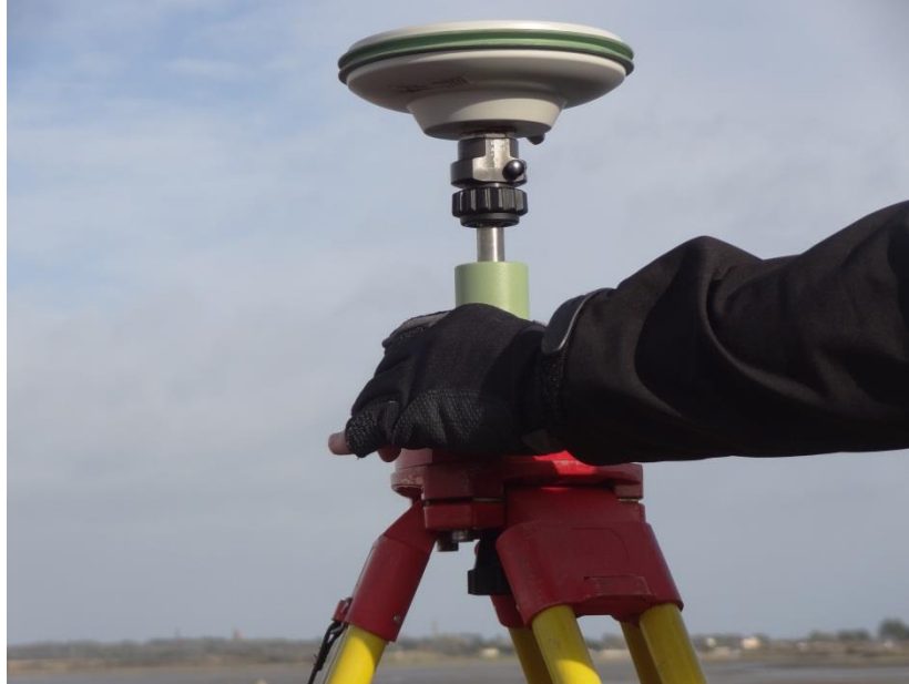
Figure 41 - GPS receiver fixed to the Tripod
