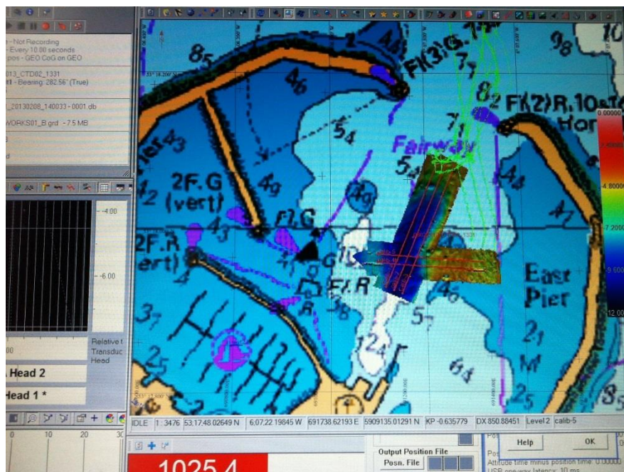
Figure 19 - Calibration lines run in DunLaoghaire at the start of survey operations
