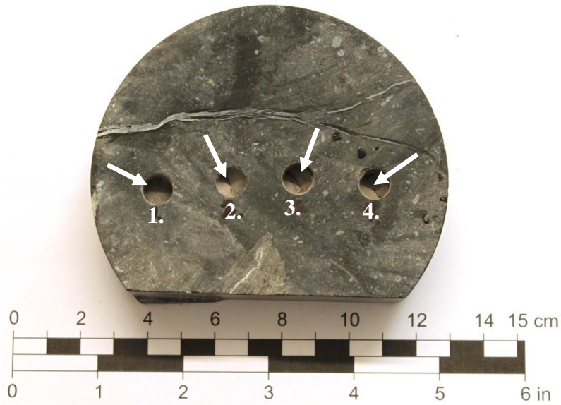
Photo of the Sievers' J (SJ) specimen subsequent to completed testing. The numbered white arrows indicate the position of the drillings.
