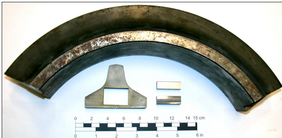
Part of a cutter ring, a 10 mm slice taken from the same ring, and two prepared AVS test pieces which are cut out of the centre of the slice.
