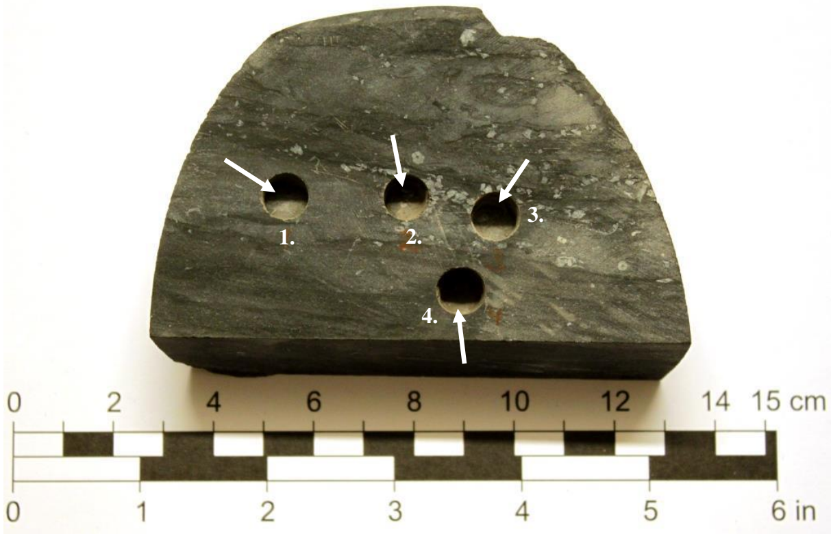
Photo of the Sievers' J (SJ) specimen subsequent to completed testing. The numbered white arrows indicate the position of the drillings.
