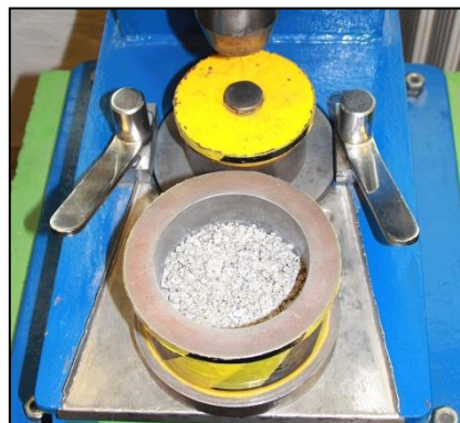
A sample subsequent to 20 impacts.
