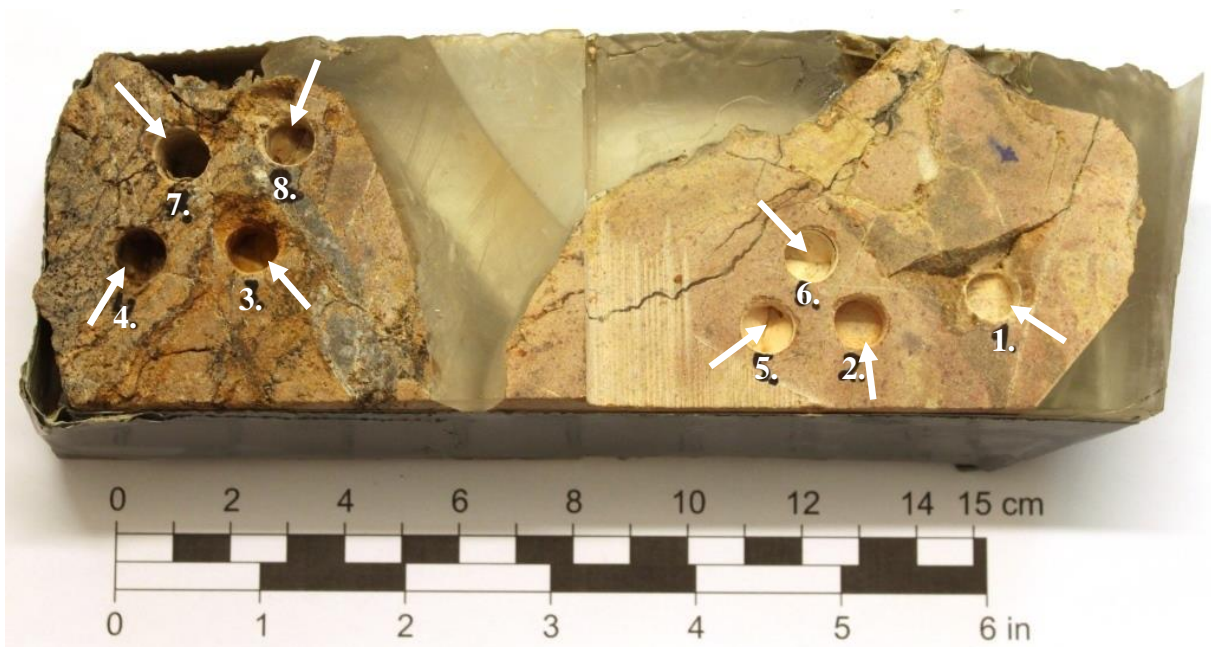
Photo of the Sievers' J (SJ) specimens subsequent to completed testing. The received sample consisted of weathered/alterd rock core sections/fragments and soil particles (see photo on page 22). It was in accordance with the Client hence decided to separate the intact rock core fragments and perform the testing on a reconstituted sample. The selected two core fragments for determination of SJ were, due to the visually observed weak texture, moulded in epoxy prior to testing in order to avoid breakage. The numbered white arrows indicate the position of the drillings.
