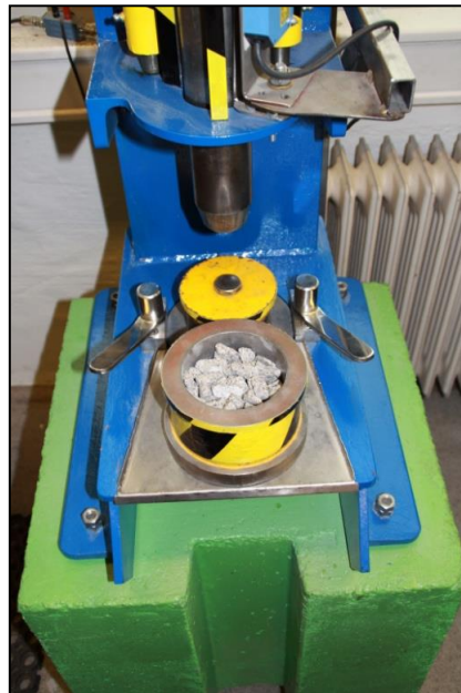
Brittleness test. Mortar with sample.
