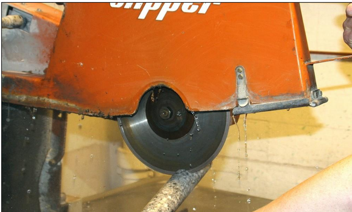
Pre-cutting of a piece from a rock core for determination of Sievers' J-Value.
