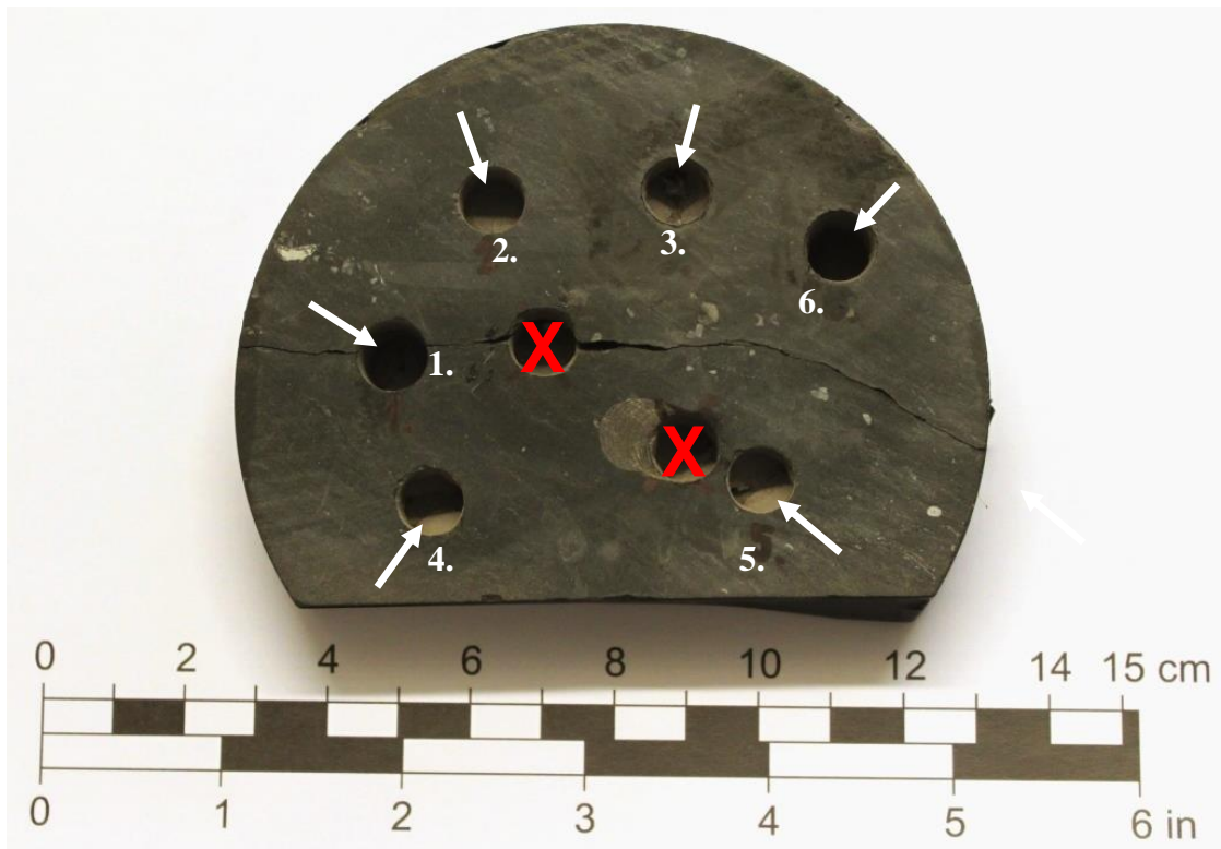
Photo of the Sievers' J (SJ) specimen subsequent to completed testing. The numbered white arrows indicate the position of the drillings. Red X indicates an unsuccessful drilling which not has been used for calculation of the SJ-Value.
