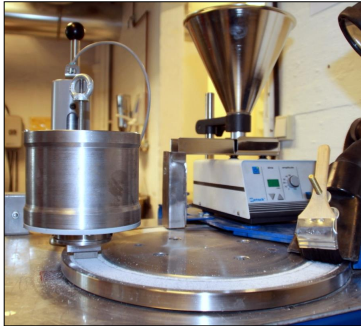
Test equipment used to determine Abrasion Value (AV) and Abrasion Value Cutter Steel (AVS).
