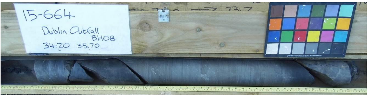
Borehole BH08 34.20 – 35.70m (photo taken after sub-sampling)
