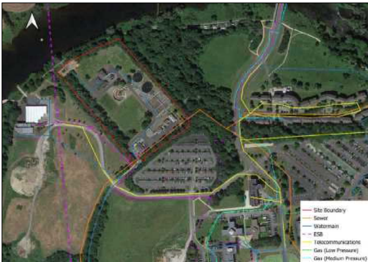
Figure 16-1: Utilities in vicinity of Proposed Development
