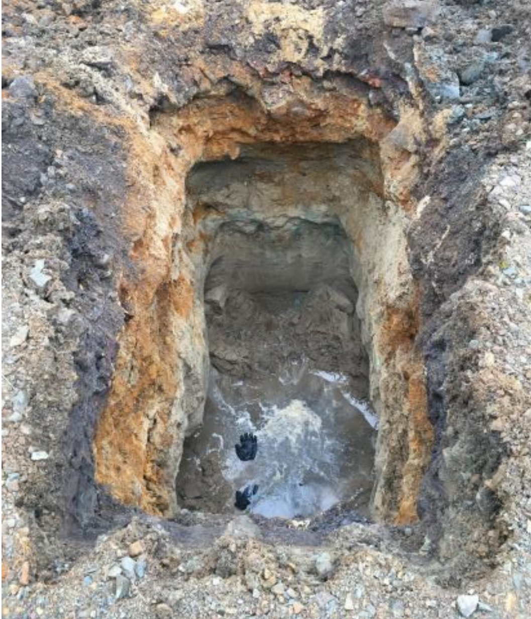
Plate 5: TP16 showing orange staining of natural deposits beneath the grey brown made ground and green staining beneath.
